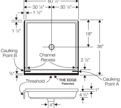
FEATURES Dimensional Tolerance ± ¼". Dimensions needed for site preparation should be measured from the unit. American Bath Group assumes no responsibility for preparatory work.
